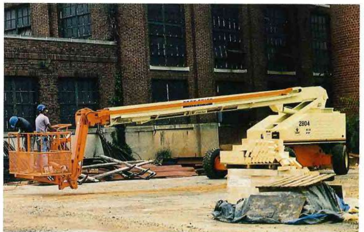
The Extend-A-Reach option articulates 15° above or 80° below horizontal of main boom to give operator "up and over" or "out and down" access.
